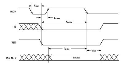
Figure 30. IDMA Write, Long Write Cycle
